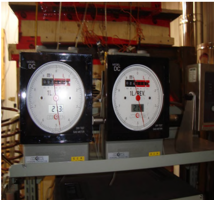
Picture 11: Dry gas meter
